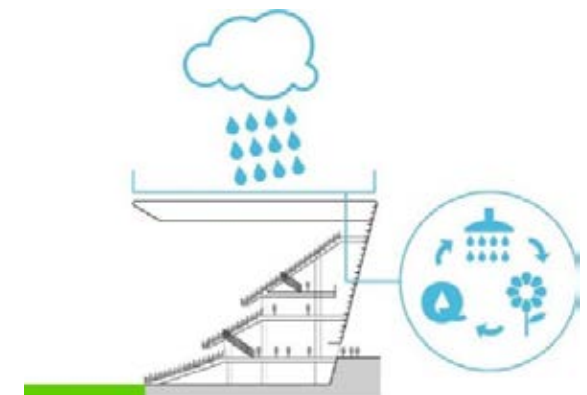
Diagram illustrating rainwater harvesting from a stadium roof
